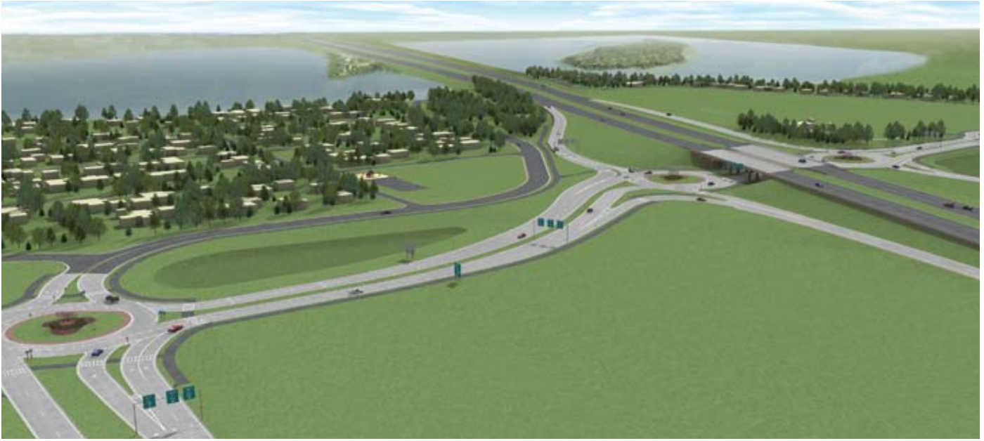
AN AERIAL PERSPECTIVE RENDERING DEPICTS PROPOSED IMPROVEMENTS, INCLUDING A SERIES OF FOUR ROUNDABOUTS AT THE I-94/COUNTY HIGHWAY P INTERCHANGE AT THE PABST FARMS DEVELOPMENT IN OCONOMOWOC, WISCONSIN.
