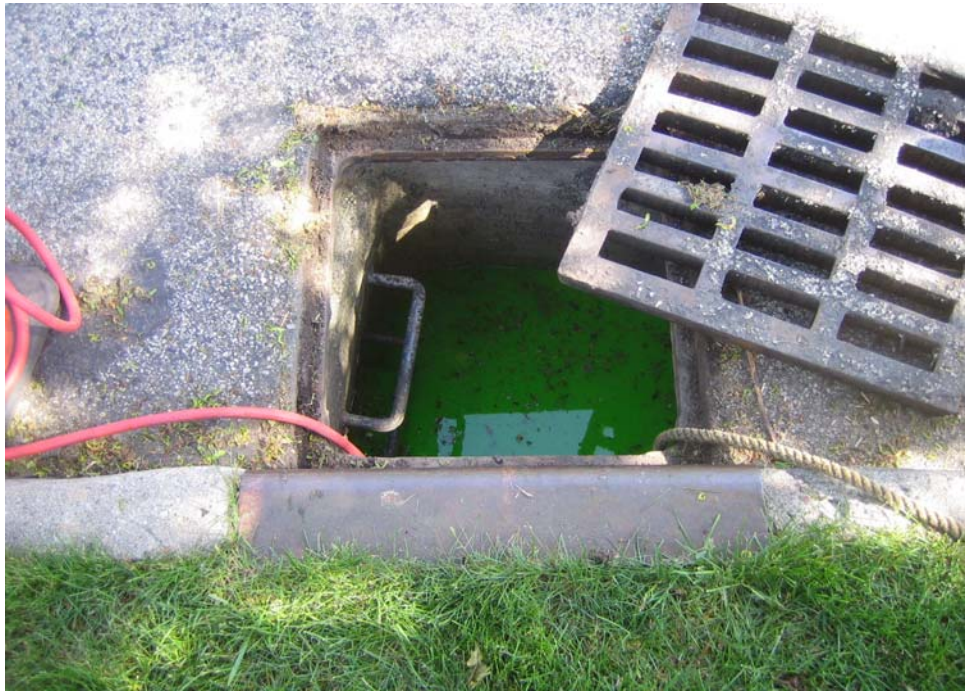
Non-toxic bright colored dye is added to a catch basin while flooding the storm sewer as part of the dye water flooding process.
