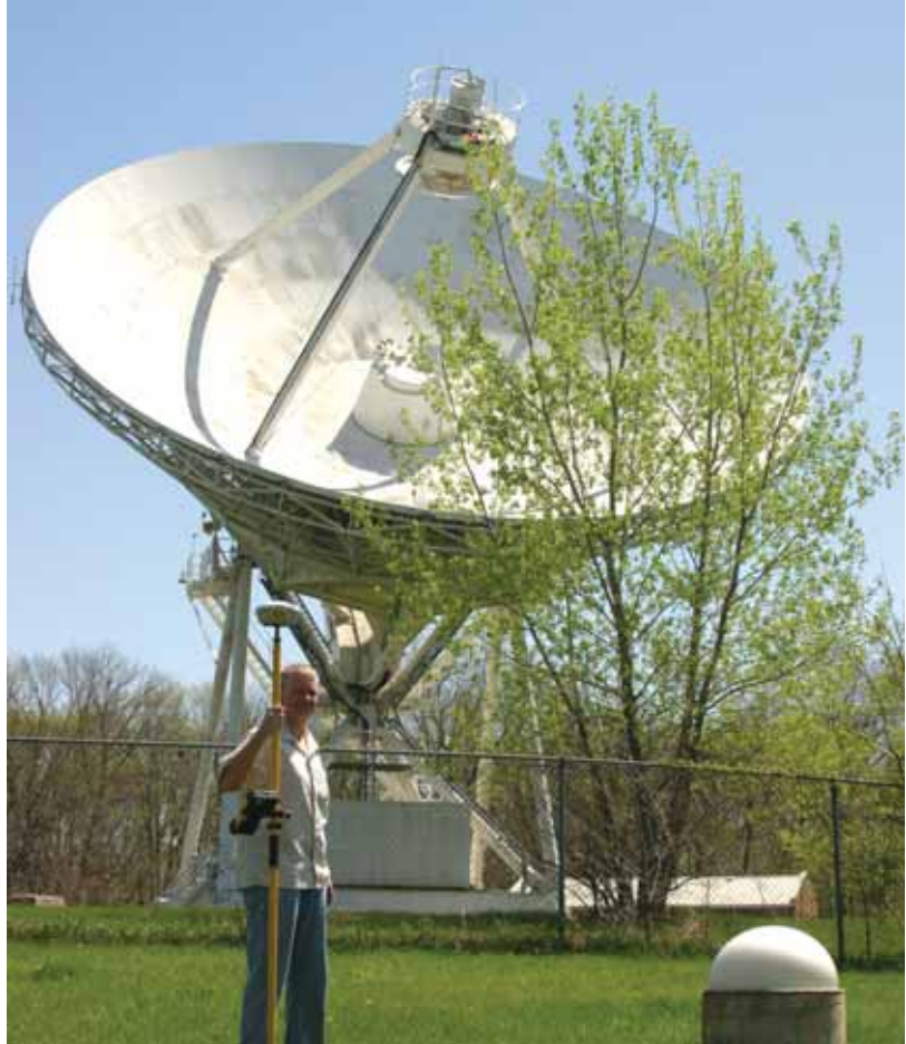
▲ This VLBI radio telescope at North Liberty, Iowa combines with other radio telescopes around the world to determine GNSS satellite orbits and give the required accuracy that makes concepts like Boundless possible. The author stands near the CORS NLIB in the foreground. —Image courtesy National Radio Astronomy Observatory
